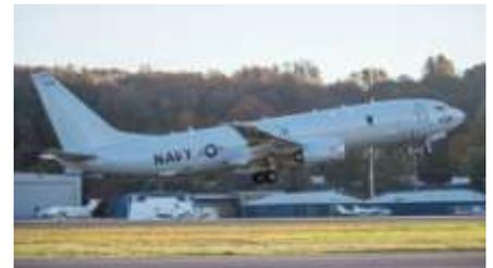
Based on Boeing's 737-800 commercial airplane, the P-8A Poseidon holds a crew of nine and can operate as an armed platform to take on targets while getting critical data to everyone on the network at the same time.
